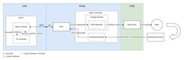
Figure 12: Diagram of SIMBA's Control Loop System.
