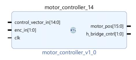
Figure 8: Single Motor Controller Verilog Module.
