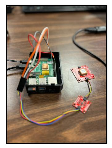
Figure 17: Test Setup of GPS (SAM\_M8Q) and IMU (ICM-20948) Module for New Code Migrations.
