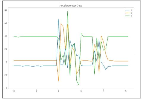
Figure 22: Accelerometer Data from IMU Displaying Acceleration of X, Y, and Z Axis in units of [m<sup>2</sup>/s].
