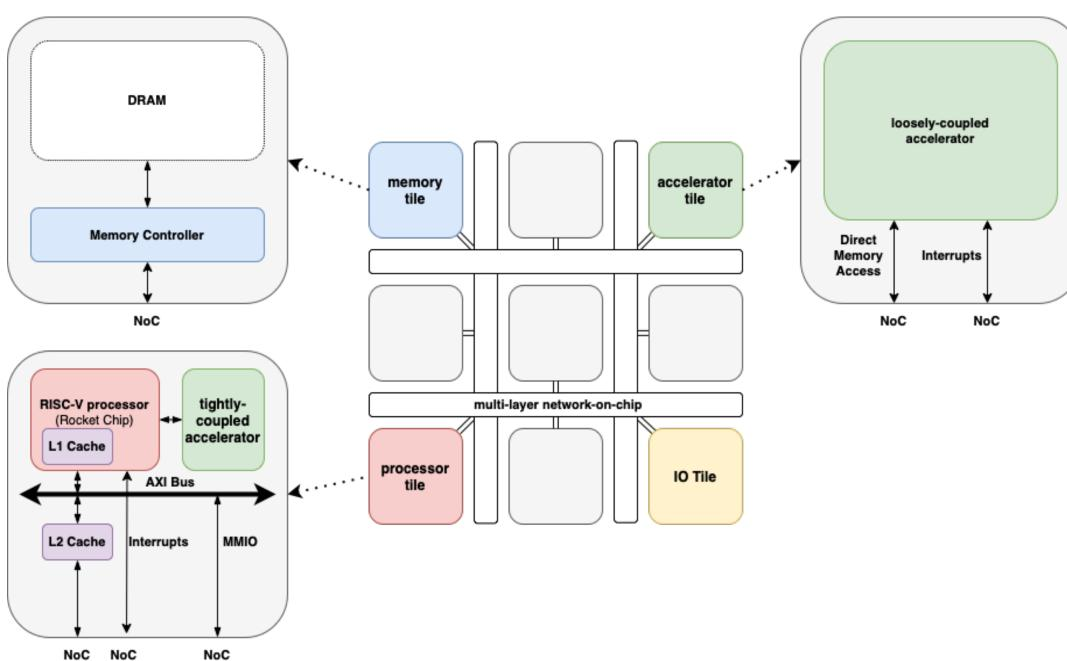
An open-source System-on-Chip design framework, surrounding modular processor, memory, IO and accelerators.
