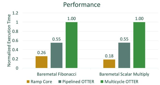
RAMP Core provides a **3x** speedup over Pipelined OTTER and over a **5x** speedup over Multicycle OTTER running bare metal benchmarks.
