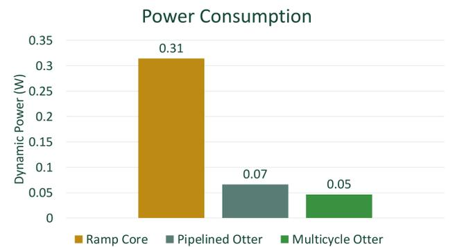
**6x** increase in power over Pipelined OTTER. Within embedded/IoT power-budget (<1W). Optimizing area and power subject for future work
